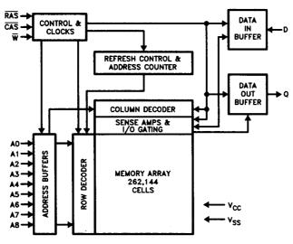
Figure 1. Functional Block Diagram
